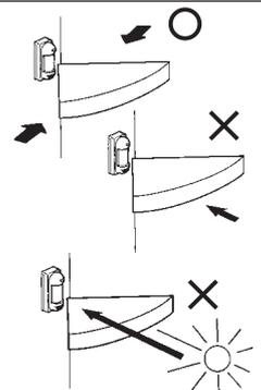
VX-402R is designed to protect any light disturbances. However , too much light such as; strong sunlight directed or reflected exactly into the sensor's field of view may cause unstable operation. It is recommended to avoid installing in such a place.
