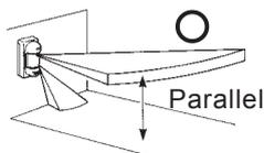
If the sensor is installed with some angle to the ground, operational reliability of the sensor may be decreased.
