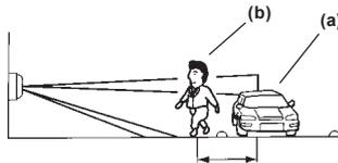
The detection area might increase when there is a big temperature difference between the moving object and the background.
