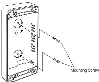
(2) Pass the wiring through the wiring port of the detector. After connecting the wires to the terminals (See 4. Wiring), insert the water protection sponge so that it blocks the wiring port as shown in the figure. Mount the detector on the back box.
