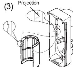
3.Put the lens back in by aligning the 4 projections on the cover to the 4 cut outs on the lens.
