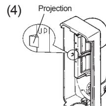
4.Mount the lens holder. make sure the lens holder is held by left and right prongs on the cover.
