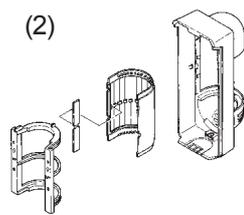
2.Separate the lens from the cover. Apply the provided area masking plate to the inside of the lens on the zone to be eliminated.
