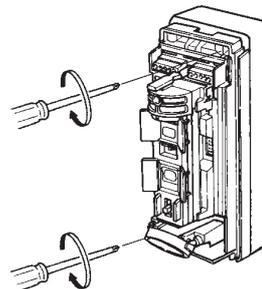
(4) Adjust the DIP switch (See 6 Switch set up), detectio area and sensitivity (See 5 Setting & Adjustment). Secure the cover with the lock screw.
