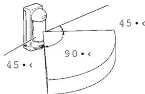
Area angle is 90degree with 7 fingers by 15degree per notch.
