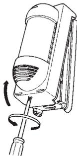
(2) Remove the screws fastening the back box.
