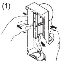
1.Remove the lens holder from the cover as shown above.
