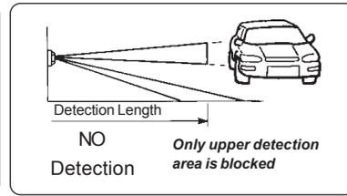
Press and slide the detection length adjustment switch to the desired position.
