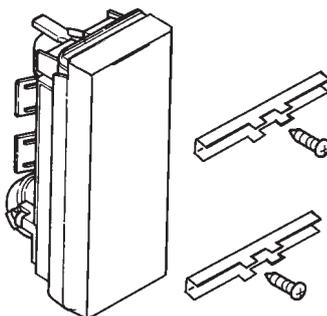
Fasten the U-brackets on the pole with the M4 x 30 screws provided. Mount in accordance with the wall mounting procedure.
