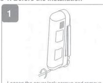
Loosen the cover lock screws and remove the front cover. Do not touch the lens surface.
